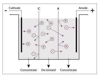
**Figure 8.10 Principle for electrodialysis.** *A and C are ion-selective membranes. In this equipment the negative ions are concentrated in the anode and the positive ions at the cathode, where they undergo electrode reactions.*
