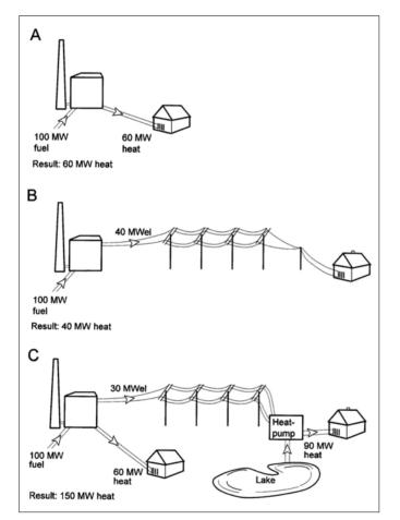
Figure 6.3 Comparison between three different alternatives for production of heating energy for households. A "bad" energy plant (A). An energy plant where all produced electricity is used for heating purposes (B), and an energy plant where the produced electricity is used to run a heat pump (C). (Illustration: Gunnar Svedberg, Royal Institute of Technology)
