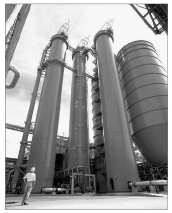
Figure 2.6 Bleaching towers in a Kraft Mill System. The sulphate process, also called the Kraft pulp process, is a recovery process, where the chemicals used in the cooking of the pulp are, generally, recycled. In addition so-called black liquor produced in the process may be incinerated and as such provide the industry with all energy needed. (Photo: @ Andritz AG)
