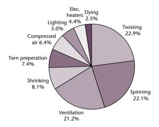
Figure 1.1 Distribution of the electricity consumption among processes and auxiliary equipment.
