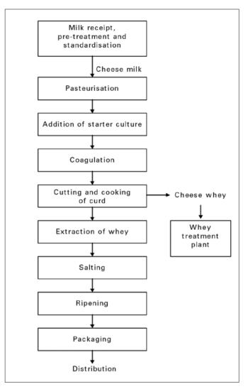
Figure 1.3 Flow diagram for a typical cheese plant.
