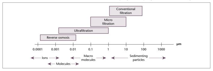
**Figure 8.9** *Classification of membrane separation processes for liquid systems according to separation ranges, here from 0.001 \mum. The measurements are approximate.*
