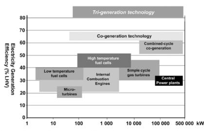
Figure 6.6 Comparison of the over-all energy efficiency between different electricity generation technologies [Adapted from brochure: Trigeneration, EPA Combined Heat and Power Partnership, 1999.].
