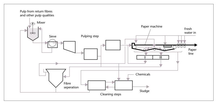
Figure 7.5 Water cycle in a mill for recycled paper.
