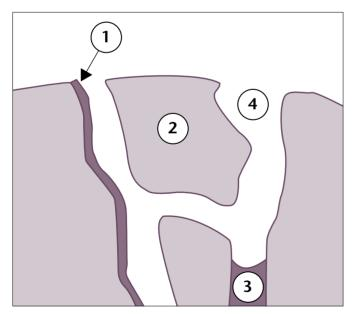
**Figure 8.3** Adsorption mechanisms in a porous adsorbent. (1) The adsorbed substance forms a monomolecular layer on the surface of the pores. (2) A small molecule penetrates into the solid phase. (3) The adsorbed substance forms a liquid plug. (4) The adsorbate is dissolved in the fluid inside the pore structure.
