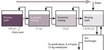
**Figure 6.5** *Comparison between different alternatives for process integration of a surface treatment process.*
