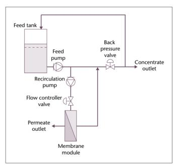
Figure 1.6 Membrane filtration with internal recirculation.
