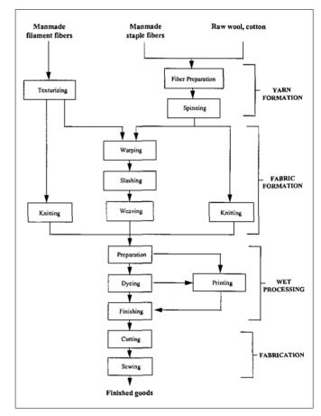
Figure 3.1 Typical textile processing flow chart [US EPA, 1997].
