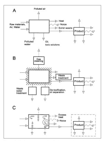
**Figure 2.1 Industry generated pollution.** *An industrial process (A) causes different kinds of pollution problems. These can be solved by external measures (B), or internal measures (C). (B) and (C) can also be combined.*
