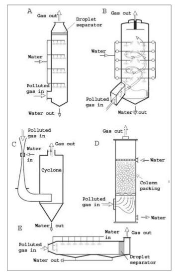
**Figure 9.5 Wet scrubbers.** Spray scrubber (A), Cyclone scrubber (B), Venturi scrubber with cyclone (C), Packed bed scrubber (D) and Cross flow spray scrubber (E).
