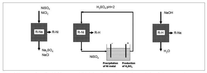
Figure 8.1 Recovery of metallic nickel from waste nickel plating solutions using ion exchange and electrolysis. Left:  $Ni^+$  in the wastewater stream is adsorbed to an ion exchanger resin (R). Middle:  $Ni^+$  is desorbed from the resin with low pH solution and precipitated as metallic nickel on the cathode of an electrolytic bath. Right: The ion exchanger is regenerated using NaOH solution.
