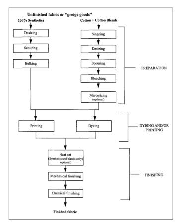
Figure 3.3 Typical wet processing steps for fabrics [ATMI, Textiles: America's First Industry, 1997].
