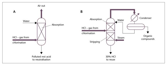
Figure 7.6 Processes for chlorinating of hydrocarbons; conventional absorption of HCl with water (A), and a new process – adiabatic absorption with evaporation (B), respectively.
