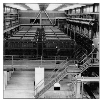
Figure 5.4 View of a membrane cell room equipped with bipolar electrolysers.
