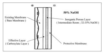
Figure 5.3 Structure of Fx-50 membrane producing 50% caustic soda.
