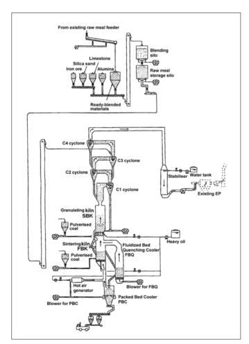
Figure 6.4 Fluidised bed cement kiln.
