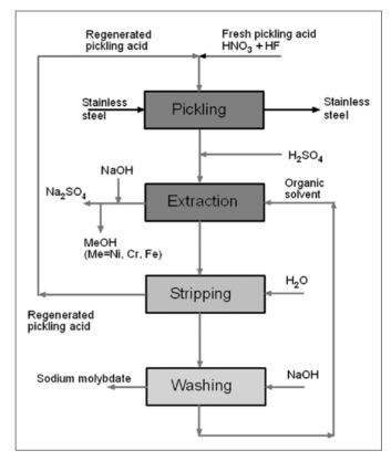
Figure 8.6 Recovery of steel mill pickling acid by extraction.
