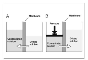
**Figure 8.4** In ordinary osmosis (A) the solvent flows form a higher to a lower concentration. In reverse osmosis (B) an external pressure forces the solvent in the opposite direction to form a more concentrated solution.
