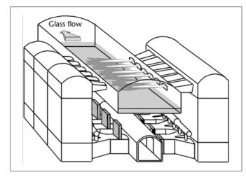
Figure 4.2 A cross-fired regenerative furnace.
