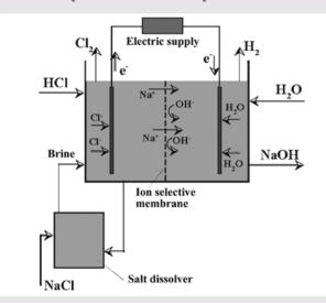
**Figure 12.1b** *The construction of a electrolysis cell for the membrane method used in the chlor-alkali process. See also the Cleaner Production Practice section.*
