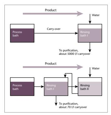
Figure 6.2 Countercurrent rinsing.
