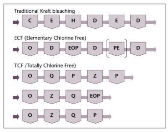
**Figure 5.2** *Examples of bleaching sequences. Bleaching chemicals are elemental chlorine (C), sodium hypochlorite (H), chlorine dioxide (D), oxygen (O), ozone (Z) and hydrogen peroxide (P). Metals are removed with a complexing agent (Q) such EDTA or DTPA [adapted from Miljöinfo från Skogsindustrierna, 1995].*
