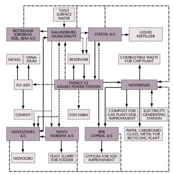
**Figure 11.2** Flow sheet of the Industrial Symbiosis of Kalundborg, Denmark. Dark colour indicates a company; lighter colour a product. [adapted from http://www.symbiosis.dk].
