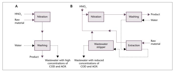
**Figure 7.7 Nitration of hydrocarbons**, an earlier process (A) and a developed process (B) which through reuse and recirculation of "rest"-products and unreacted raw material leads to a decreased environmental hazard potential in the wastewater.
