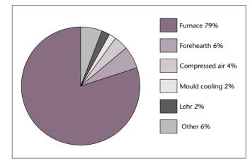
Figure 4.3 Energy usage in a typical container glass plant.
