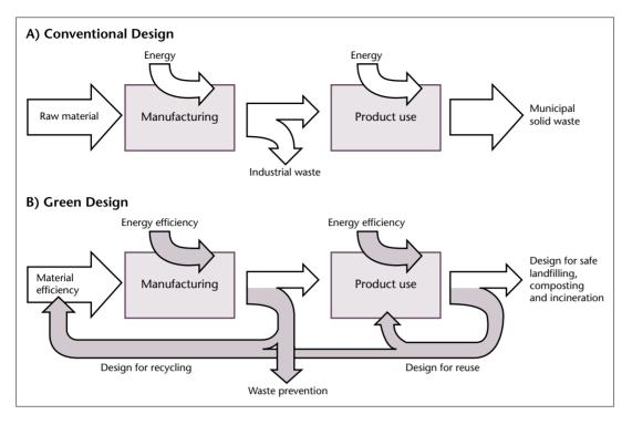
Figure 11.1 How product design affects material flows. Making changes in a product's design reduces overall environmental impact. The green design emphasises the efficient use of material and energy, reduction of waste toxicity, and reuse and recycling of materials. [Reprinted from OTA, 1992].
