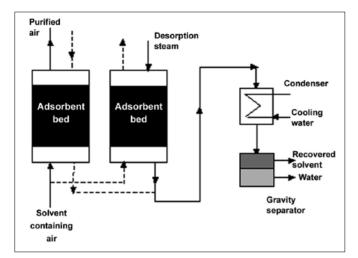
**Figure 9.3** Adsorption of a polluting solvent in exhaust air (left) in fixed bed columns. The adsorbent, typically activated carbon, is packed in columns (adsorbent beds). In a second step (right) the solvent is desorbed from the saturated column with steam and condensed to liquid phase and separated from water by settling (far right). While one column is used for adsorption the second is washed (dotted lines) and vice versa which makes continuous operation possible.
