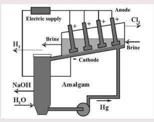
**Figure 12.1a** *The construction of an electrolysis cell for the mercury method used in the chlor-alkali process. See also the Cleaner Production Practice section.*
