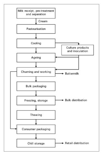
Figure 1.2 Flow diagram for a typical butter-making plant.
