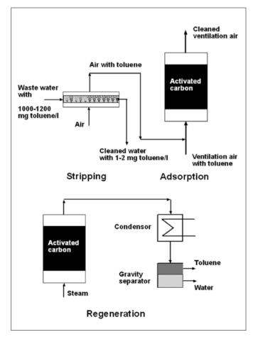
Figure 8.7 Recovery of toluene from printing wastewater.
