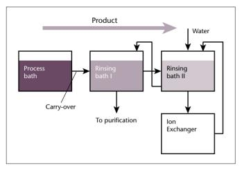
Figure 6.4 Ion exchange as a kidney stage.
