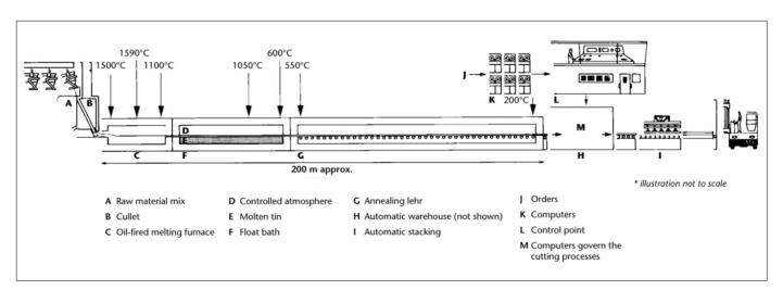
Figure 4.1 The float glass process.
