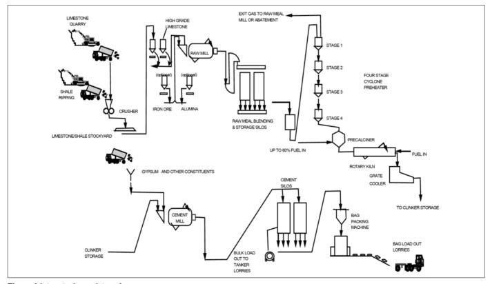
Figure 6.1 A typical precalciner dry process.
