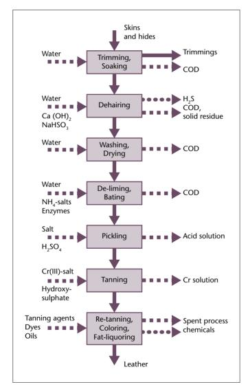
Figure 12.3 Process flow diagram of leather tanning using chromium III as the tanning agent [UNEP, 1996].
