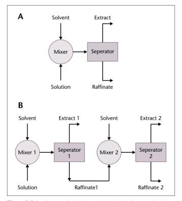
**Figure 8.5** *Single-stage batch extraction (A) the solvent and solution is mixed and later separated to allow the purified raffinate to continue, while the pollutant is found in the extract. In a two (B) or multi-stage extraction the procedure is repeated to achieve a more efficient purification.*
