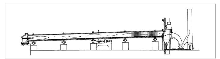
Figure 6.2 Long wet rotary kiln with chains.
