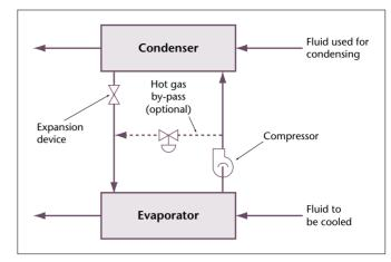
Figure 6.11 Vapour-compression refrigeration system [Perry and Green, 1984].
