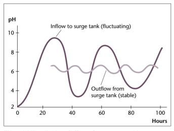
**Figure 8.2 Equalisation of effluent from a process using a surge tank.** *The inflow waste stream to the tank has large variation of pH due to the cyclic nature of the process, while the outflow has less variation as pH is equalised in the tank. The volume of the tank should correspond to at least one cycle [Nemerow and Dasgupta, 1991].*
