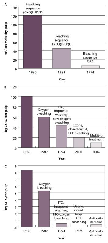
**Figure 5.4** *A)* Wastewater flows, total volume from SCA Forest Products, Östrand pulp mill. B) COD in the wastewater. C) AOX in the wastewater. Bleaching sequences are shown in Figure 5.2.
